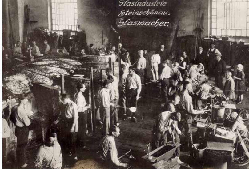
Kamenický Šenov, glassworks complex, house No. 687, view into the interior of the glassworks hall with a Siemens-Siebert melting furnace. Stanislav Kopecký's collection.
