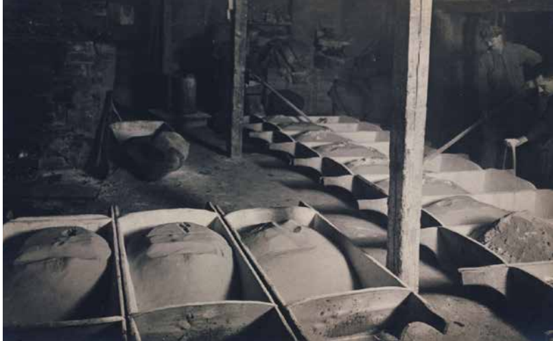
Interior of the mixing chamber with wooden troughs for mixing the glass mixture. Petr Joza's collection.
