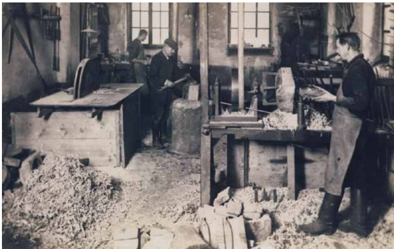
Interior of the form works with the production of wooden glass forms. Petr Joza's collection.
