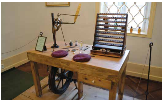
Model of an engraving machine with foot propulsion, exposition of the Glass Museum Kamenický Šenov. Photo: author, 2022.
