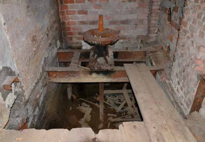
Lindava, mirror grinding and polishing works, house No. 308, torso of the transmission mechanisms from the turbine in the engine room on the ground floor next to the rock waterwheel chamber. Photo: author, 2020.
