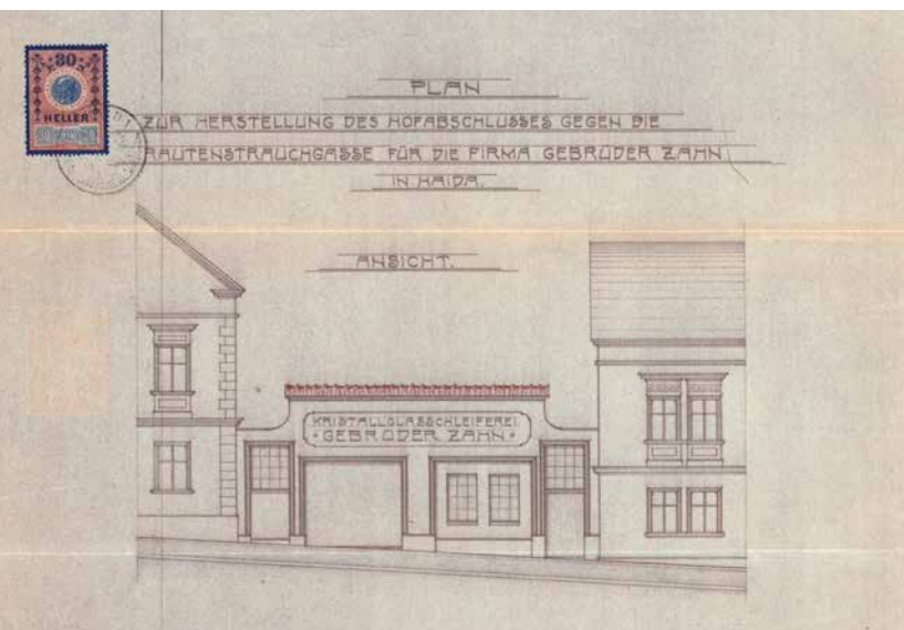
Nový Bor, Gebrüder Zahn finishing plant; plan of the construction of a preserved enclosure wall with a gate between houses No. 320 and 315 (1903, Maxmilian Dittrich, Nový Bor). Nový Bor Building Authority, file of house No. 320.
