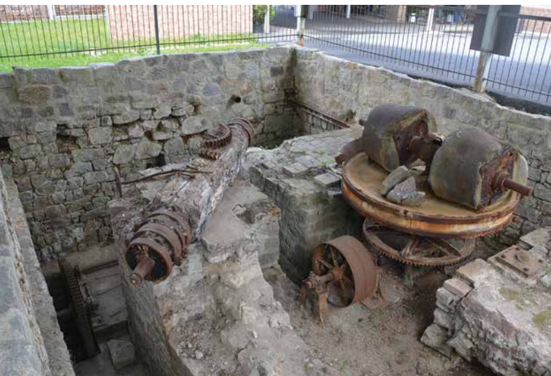
Harrachov, Nový Svět glassworks, view of the uncovered relics of a stamp battery, house No. 87; a wheel mill on the right, a shaft on the left, and transmission mechanisms leading from the waterwheel chamber (outside the photograph to the left) in the bottom. Photo: Ivan Peřina, 2013.
