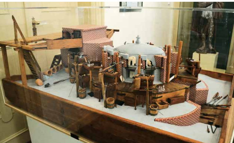
Model of a Bohemian glass furnace from the Preitenstein glassworks near Nečtiny, F. Rückl, c. 1850, exposition of the Glass Museum Kamenický Šenov. Photo: author, 2022.
