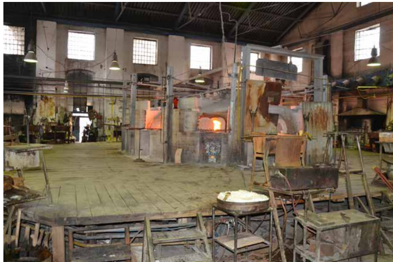
Nový Bor, Florahütte glassworks, house No. 399; view of the melting furnace heated by natural gas in the old glassworks hall, which has a new steel roof structure after reconstructions. Photo: author, 2018.
