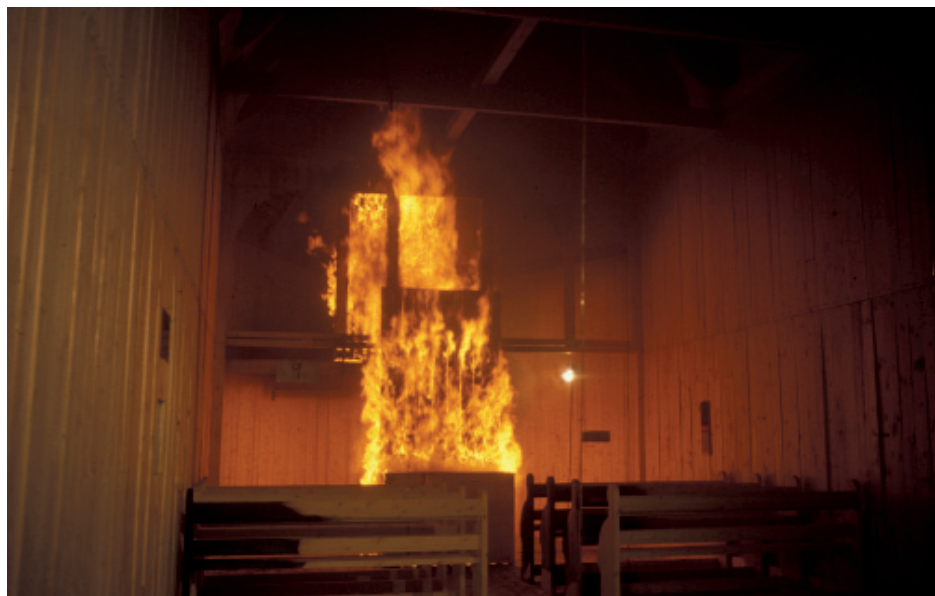
Test of water mist in a mock-up of a stave church
